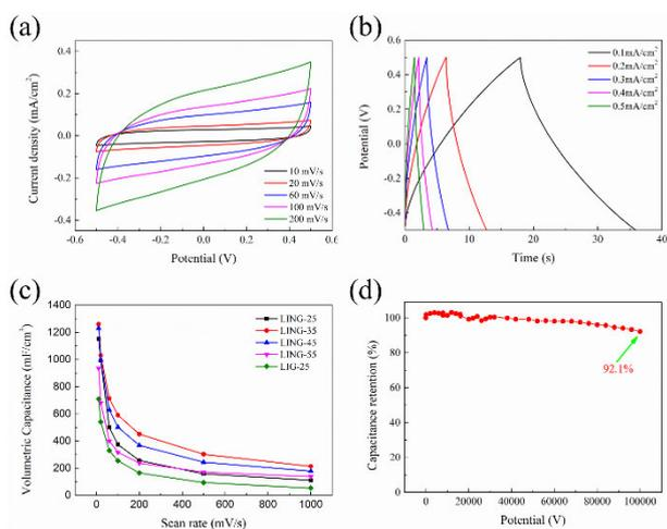
Fig. 3. CV (a) and GCD (b) results of LING-35 at different conditions. (c) The volumetric capacitance of LING-25, LING-35, LING-45, LING-55, LING-25 at different scan rates. (d) Cycling stability of LING-35.
