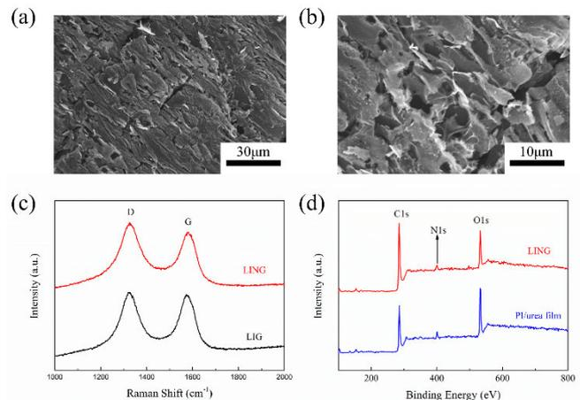
Fig. 2. SEM image of LING after laser direct writing at low (a) and high (b) magnification. (c) Raman spectrums of LING and LIG. (d) XPS spectra of LING.
