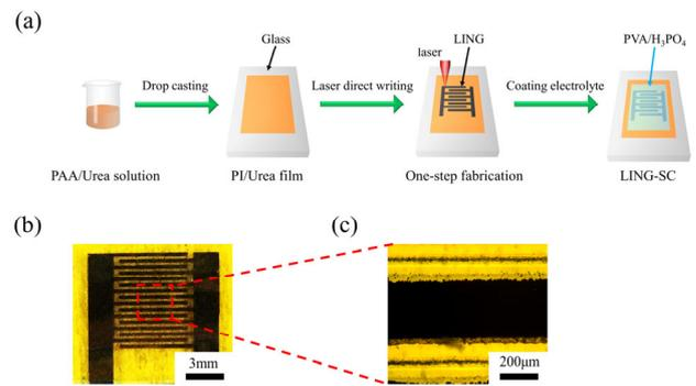
Fig. 1. (a) Fabrication process of LING. Optical photograph of LING-SC at low (b) and high (c) magnification.
